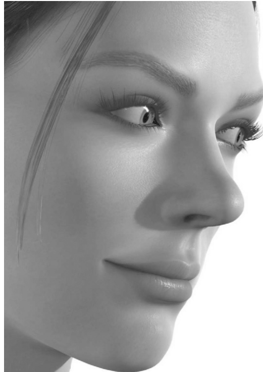
FIGURE B.3.2 GPU-rendered image. To give the skin visual depth and translucency, the pixel shader program models three separate skin layers, each with unique subsurface scattering behavior. It executes 1400 instructions to render the red, green, blue, and alpha color components of each skin pixel fragment.
