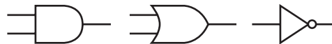
FIGURE A.2.1 Standard drawing for an AND gate, OR gate, and an inverter, shown from left to right. The signals to the left of each symbol are the inputs, while the output appears on the right. The AND and OR gates both have two inputs. Inverters have a single input.
