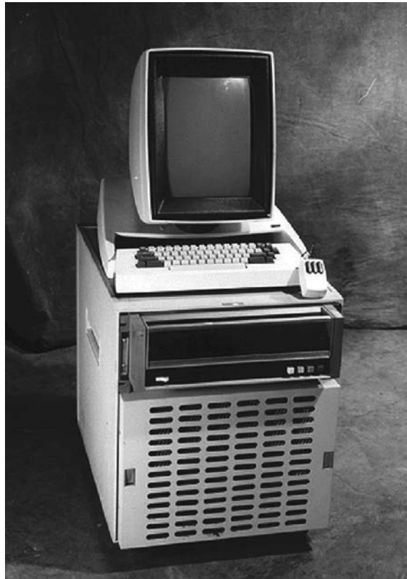
FIGURE e1.13.6 The Xerox Alto was the primary inspiration for the modern desktop computer. It included a mouse, a bit-mapped scheme, a Windows-based user interface, and a local network connection.
