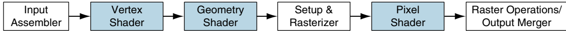
FIGURE B.2.3 Graphics logical pipeline. Programmable graphics shader stages are blue, and fixed-function blocks are white.
