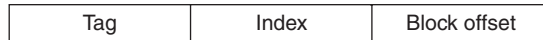
FIGURE 5.17 The three portions of an address in a set-associative or direct-mapped cache. The index is used to select the set, then the tag is used to choose the block by comparison with the blocks in the selected set. The block offset is the address of the desired data within the block.
