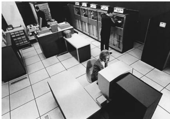
FIGURE e1.13.3 IBM System/360 computers: models 40, 50, 65, and 75 were all introduced in 1964. These four models varied in cost and performance by a factor of almost 10; it grows to 25 if we include models 20 and 30 (not shown). The clock rate, range of memory sizes, and approximate price for only the processor and memory of average size: (a) model 40, 1.6 MHz, 32 KB–256 KB, $225,000; (b) model 50, 2.0 MHz, 128 KB–256 KB, $550,000; (c) model 65, 5.0 MHz, 256 KB–1 MB, $1,200,000; and (d) model 75, 5.1 MHz, 256 KB–1 MB, $1,900,000. Adding I/O devices typically increased the price by factors of 1.8 to 3.5, with higher factors for cheaper models.
